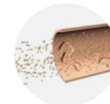
Corroded pressure pipes are blasted with garnet to prepare them for the rehabilitation process
